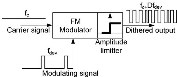
Figure 4. Simplified equivalent model of the dithered output generation.
