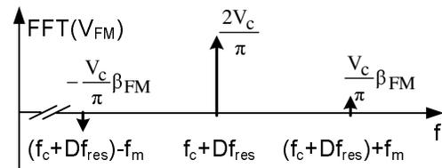
Figure 8. Spectral content of NBFM representation of the dithered output.
