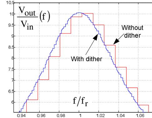
Figure 3. Simulated frequency response (sweep) of a resonant network, with DPWM frequency steps and proposed method.
