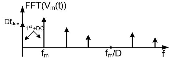
Figure 7 Typical Spectral content of the dithered signal of Fig. 6
