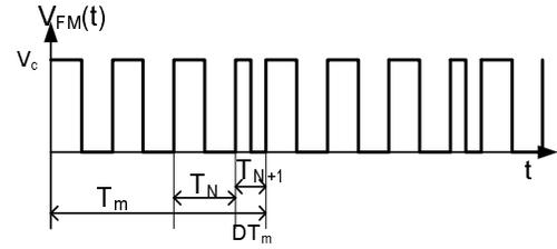
Figure 1. Dithered drive signal with frequency fraction of  $0.25f_{res}$ .
