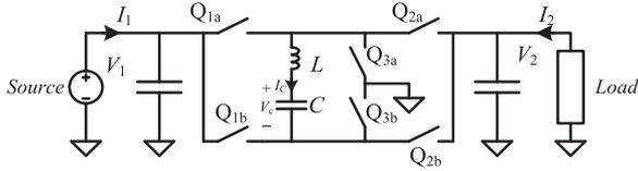
Fig. 2. Multimode switched-resonator converter.
