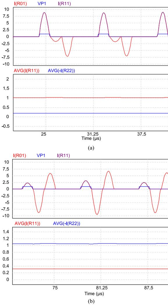
Fig. 4. PSIM simulation of the sequence:  $\{V_{in}, V_{out}, 0\}$  for two cases: (a)  $V_{in} = 5\text{ V}$ ,  $V_{out} = 20\text{ V}$ . (b)  $V_{in} = 20\text{ V}$  and  $V_{out} = 5\text{ V}$ . Upper traces: Resonator current (0.5 A/div.) while the pulse indicates the switching duration of  $V_{in}$ . Lower screens: Average currents for the voltage sources  $V_{in}$  and  $V_{out}$  (0.5 A/div.), higher current corresponds to the lower voltage.
