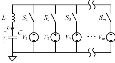
Fig. 1. Simplified model representation of a generic switched-resonator converter with  $m$  switched-source ports.
