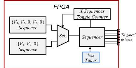
Fig. 7. Block diagram of the driving sequencer of the experiment.
