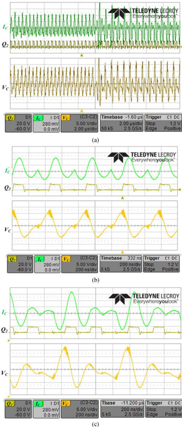
Fig. 8. Experimental results of the sequences  $V_1$ ,  $V_2$ , 0 and  $\{V_1, V_2, 0, V_2, 0\}$ . In each screen, the upper trace is the resonator's current (relative scale) and the lower trace is the capacitor's voltage (5 V/div.). (a) Behavior when the two sequences are run in tandem. (b) Zoom on the three switching states case. (c) Zoom on the five switching states case.
