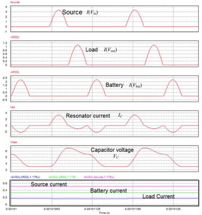
Fig. 6. Simulation results of the DC UPS. Traces: From up to down,  $V_{in}$  current,  $V_{load}$  current,  $V_{bat}$  current, resonator current, capacitor voltage. Lower screen, average currents for the voltage sources  $V_{in}$  (upper trace),  $V_{bat}$  (middle trace),  $V_{load}$  (lower trace).
