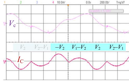
Fig. 3. Waveforms of the even case sequence:  $\{-V_2, V_1 - V_2, V_2, -V_1 + V_2\}$  where (19) holds. Upper trace: Resonator capacitor voltage (5 V/div), lower trace: Resonator's current (10 A/div). Horizontal scale: 200 ns/div.
