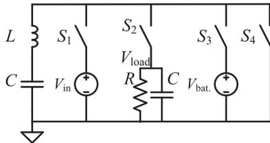
Fig. 5. Conceptual representation of a proposed switched-resonator UPS topology.
