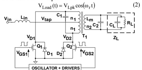
Figure 1. Basic configuration of the CFPPRI loaded by a capacitive load.
