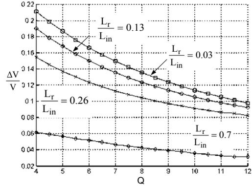
Figure 5. Output voltage sag for a 100% to 60% step of the load as a function of Q for several ratios of K ( $L_r/L_{in}$ ).
