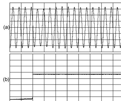
Figure 8. Response of experimental unit to a step from 60% to 100% of the output power. (a) output voltage, 70V/div and (b)  $V_{GS}$  of  $Q_L$  of Fig. 2, 5V/div ;horizontal scale: 20 $\mu$ s/div.
