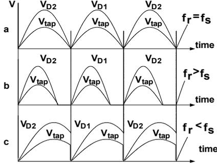
Figure 2. Drain voltages ( $V_D$ ) and tap voltage ( $V_{tap}$ ) when the gate-drive frequency matches the resonant frequency (a) and when it is lower (b) or higher (c) than the resonant frequency
