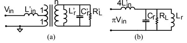
Figure 3. CFPPRI simplified circuit. (a) One-half cycle operation and (b) reflected to the primary.
