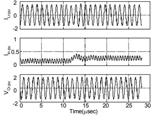
Figure 4. Cycle-by-cycle step response waveforms, the load is switched from 100% to 60%.
