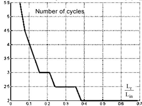
Figure 6. Number of switching cycles that passes from a step perturbation of the load to overshoot of the output voltage as a function of K ( $L_r/L_{in}$ ).
