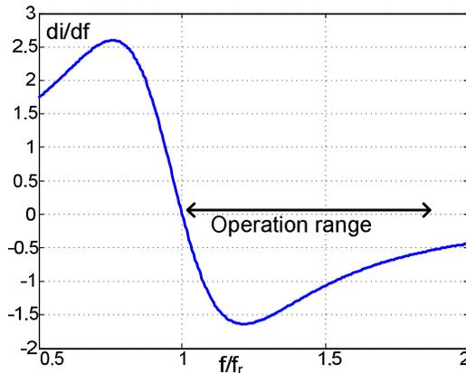
Figure 5. Normalized frequency sensitivity of the resonant current.
