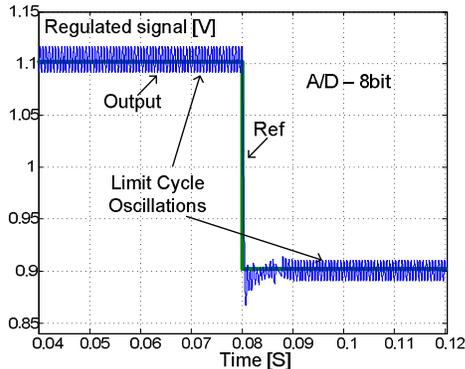
Figure 8. Simulation results of the model of Fig. 7 for a step of current amplitude from 1.1 to 0.9 (arbitrary units), ADC level of 8bit. Limit cycle oscillations.
