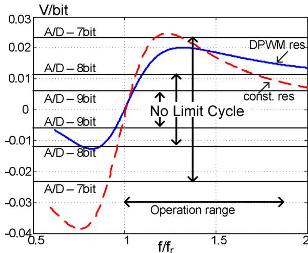
Figure 6. System frequency sensitivity. Map of no-limit-cycle operation conditions for the system of Fig. 2
