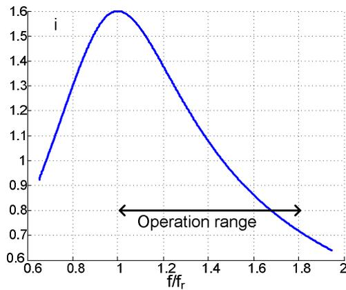
Figure 4. Normalized frequency response of the power stage of Fig. 2.
