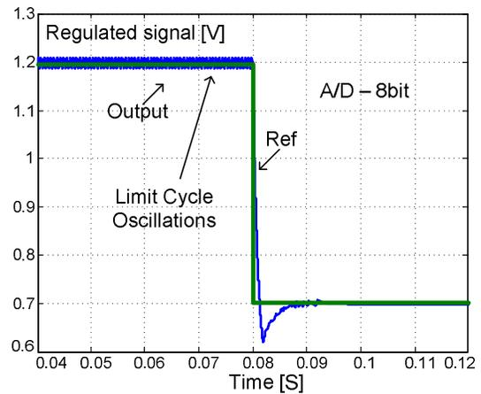
Figure 10. Simulation results of the model of Fig. 7 for a step of current amplitude from 1.2 and 0.7 = ADC level of 8bit. Limit cycle oscillation at 1.2 and no oscillations at 0.7.
