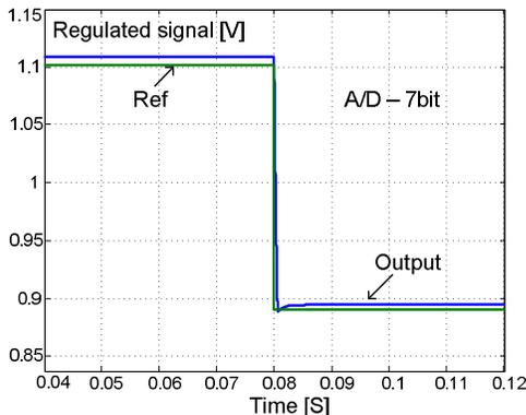
Figure 9. Simulation results of the model of Fig. 7 for a step of current amplitude from 1.1 to 0.9 (arbitrary units), ADC level of 7bit. Free of limit cycle oscillations.
