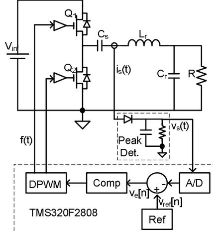
Figure 2. The experimental digitally controlled series-resonant parallel-loaded converter.
