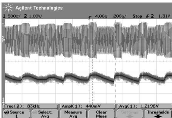
Figure 11. Experimental results of the converter of Fig. 2. For current amplitude at 0.15A with 9bits ADC, limit cycles. Upper trace: resonant current 0.2A/div, lower trace: peak detector output 0.5V/div. Horizontal scale 200µS/div.
