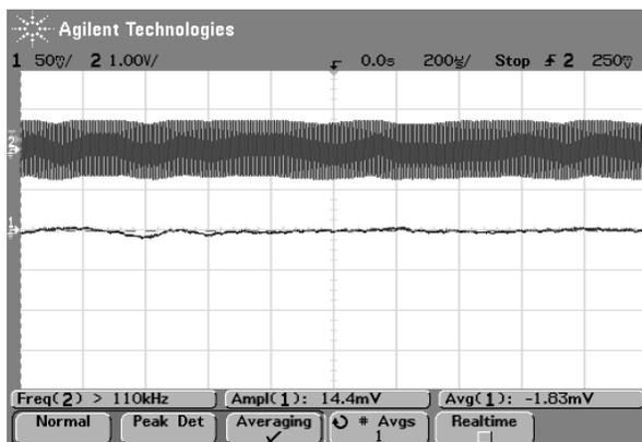
Figure 12. Experimental results of the converter of Fig. 2 for a current amplitude of 0.15A with 7bits ADC. Stable steady state operation. Upper trace: resonant current 0.2A/div, lower trace: peak detector output 50mV/div. Horizontal scale 200µS/div.
