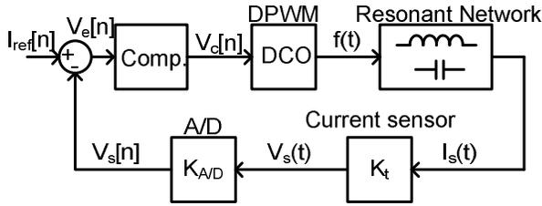
Figure1. Block diagram of a digitally controlled resonant converter
