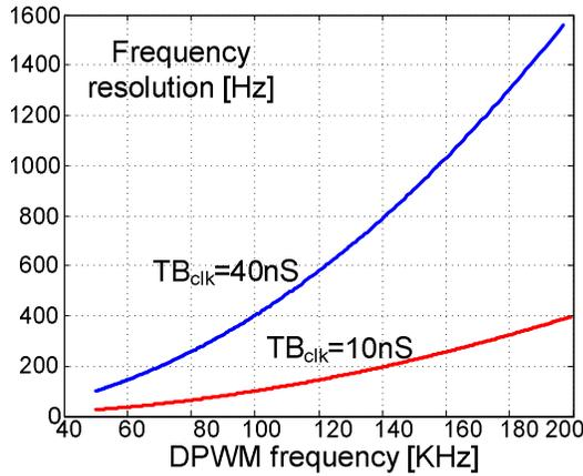
Figure 3. Frequency resolution as a function of the running frequency of typical DPWM unit for two cases of clock frequency.
