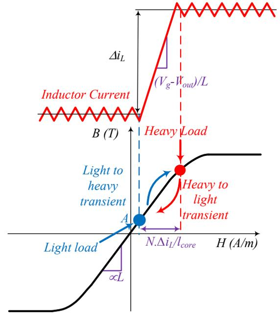
Fig.2 (a) Inductor current of a conventional buck during a light-to-heavy load transient. (b) Corresponding B-H curve with load transient trajectories; where  $L$  is inductance,  $l_{core}$  is core length,  $N$  is number of turns in the winding and  $\Delta i_L$  is the change of load current.
