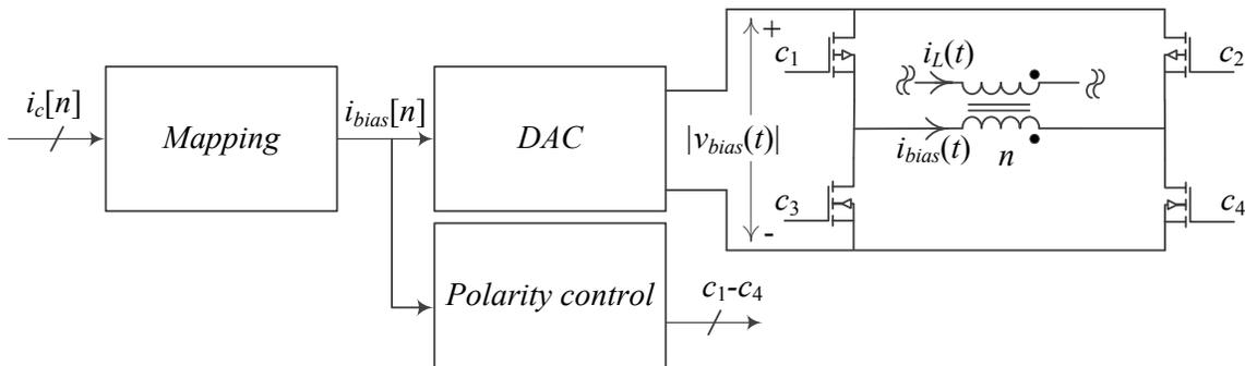
Fig.5 Low-power biasing circuit
