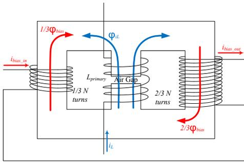
Fig.6. Implementation of the inductor with biasing winding.
