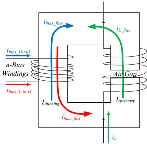
Fig.4. Simplified diagram of the inductor with biasing windings
