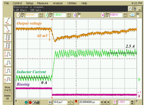
Fig.8. The light-to-heavy load transient with core biasing– Ch1: output converter voltage (50mV/div); Ch2: inductor current (1A/div).
