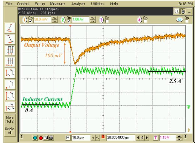
Fig.7. The light-to-heavy load transient without core biasing– Ch1: output converter voltage (50mV/div); Ch2: inductor current (1A/div).
