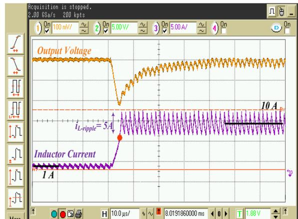
Fig.9. 9A load step without core biasing– Ch1: output converter voltage (100mV/div); Ch2: inductor current (5A/div).
