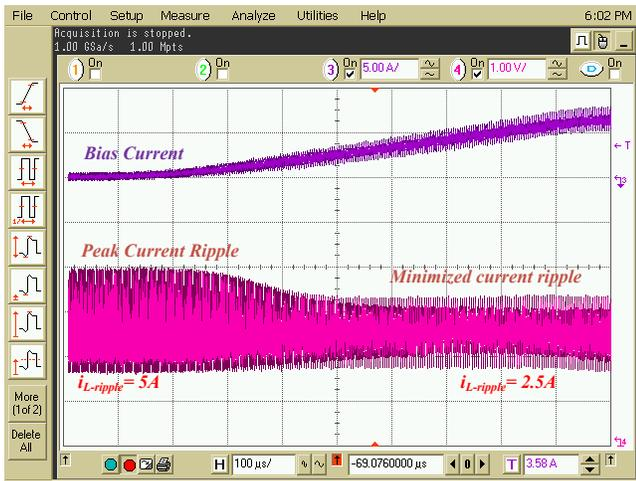
Fig.10. Inductor ripple reduction using biasing—Ch3: Bias current (5A/div); Ch4: current ripple 2A/div.
