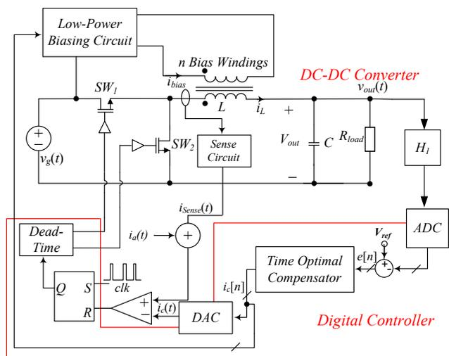
Fig. 1: Digitally-controlled buck converter with adaptive inductor biasing.
