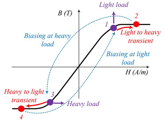
Fig.3. Relocation of the operating point on B-H curve through adaptive core biasing
