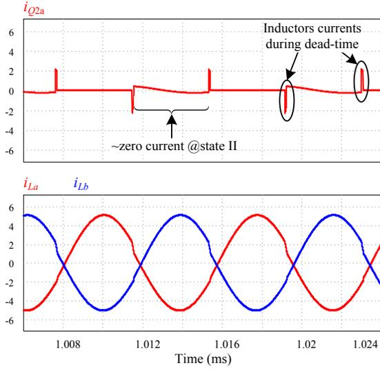
Fig. 6. Zero current characteristic of  $Q_{2a}$ .
