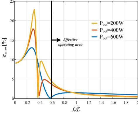
Fig. 5. Current error between the phases as a function of the switching frequency for  $C_{rb}=1.2C_{ra}$ .
