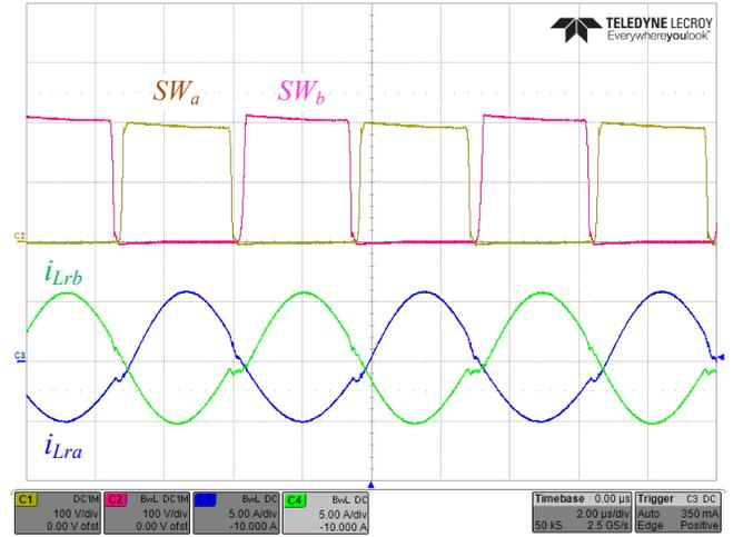
Fig. 9. Experimental waveforms of the TIFLLC converter. C1 – switching node voltage of phase  $a$   $SW_a$  (100V/div), C2 – switching node voltage of phase  $b$   $SW_b$  (100V/div), C3 – phase  $a$  primary-side resonant tank current  $i_{Lra}$  (5A/div), C4 – phase  $b$  primary-side resonant tank current  $i_{Lrb}$  (5A/div). Time scale is 2 $\mu$ s/div.
