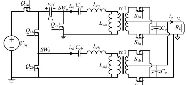
Fig. 1. Two-phase interleaved flying-capacitor LLC (TIFLLC) converter topology.
