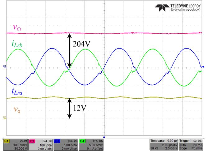
Fig. 7. Experimental waveforms of the TIFLLC converter. C1 – output voltage  $v_o$  (5V/div), C2 – flying-capacitor voltage  $v_{Cf}$  (100V/div), C3 – phase  $a$  primary-side resonant tank current  $i_{Lra}$  (5A/div), C4 – phase  $b$  primary-side resonant tank current  $i_{Lrb}$  (5A/div). Time scale is 2 $\mu$ s/div.
