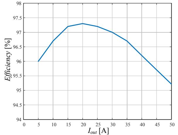
Fig. 10. Efficiency measurements of the experimental prototype.
