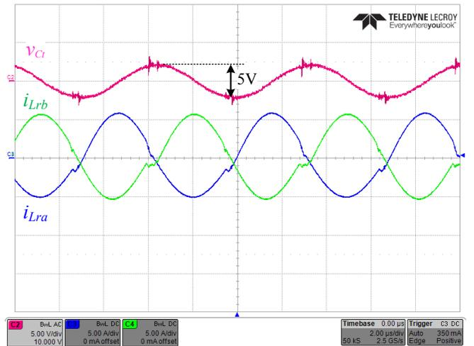
Fig. 8. Experimental waveforms of the TIFLLC converter. C2 – flying-capacitor voltage  $v_{Cf}$  (5V/div, ac coupled), C3 – phase  $a$  primary-side resonant tank current  $i_{Lra}$  (5A/div), C4 – phase  $b$  primary-side resonant tank current  $i_{Lrb}$  (5A/div). Time scale is 2 $\mu$ s/div.
