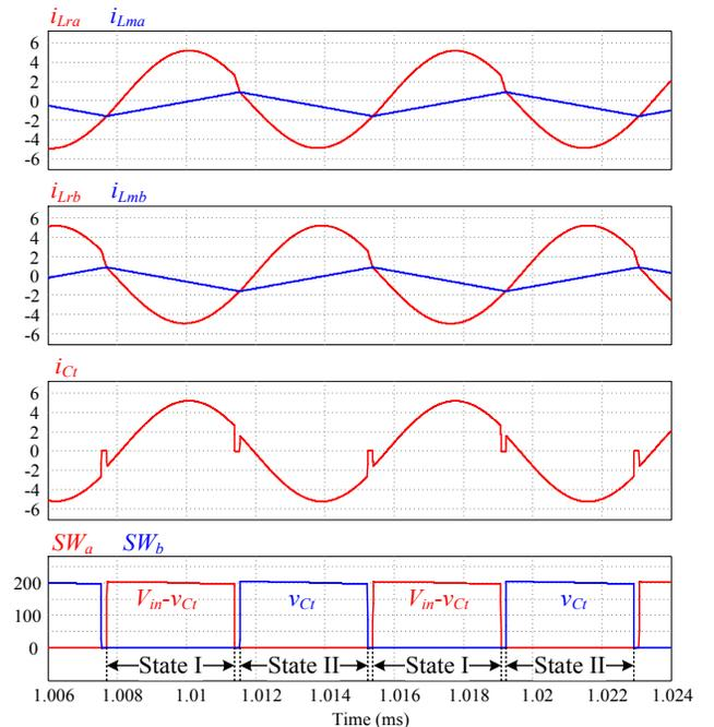
Fig. 3. Typical waveforms of the TIFLLC converter.
