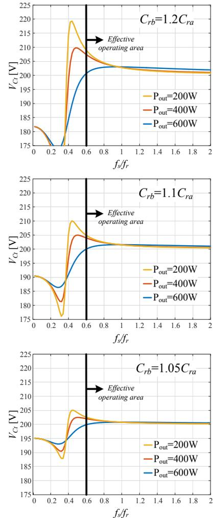
Fig. 4. Flying-capacitor voltage as a function of the switching frequency for phases with different resonant capacitors.
