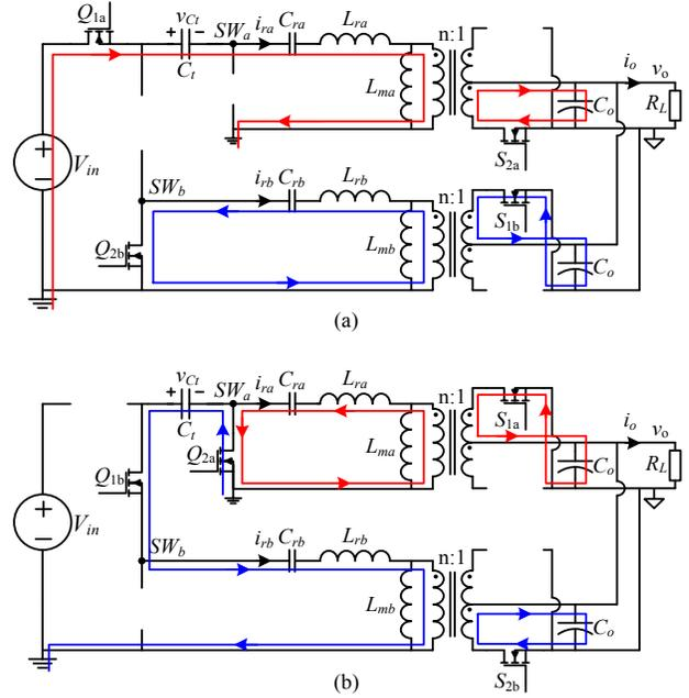
Fig. 2. Current paths in the TIFLLC converter: (a) State I: phase  $a$  is on and phase  $b$  is off, (b) State II: phase  $a$  is off and phase  $b$  is on.
