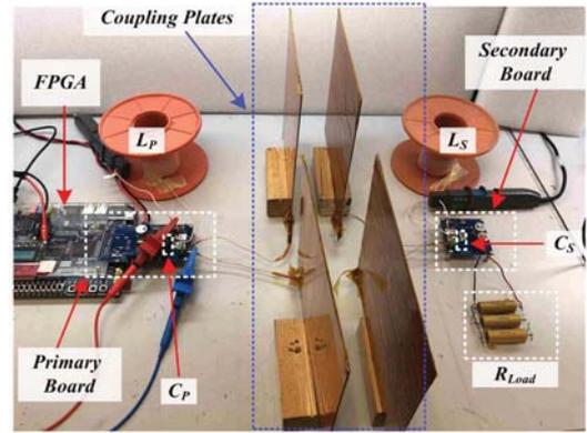
Fig. 10 Experimental setup of a double-sided LC capacitive WPT prototype.
