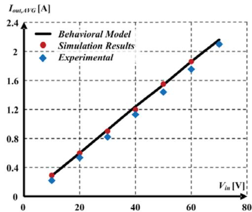
Fig. 12 Average output current,  $I_{out,AVG}$ , curve as function of the input voltage.
