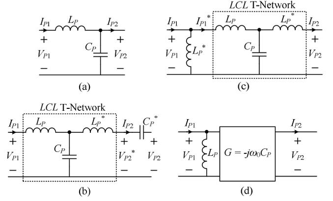
Fig. 3. Equivalent representations of series-parallel  $LC$  matching network: (a) L-type series-parallel resonant  $LC$  circuit; (b) Series resonator connected to the L-type circuit for T-type network arrangement; (c) Modified T-type series-parallel  $LC$  resonant circuit; (d) Two-port representation of the original L-type network.
