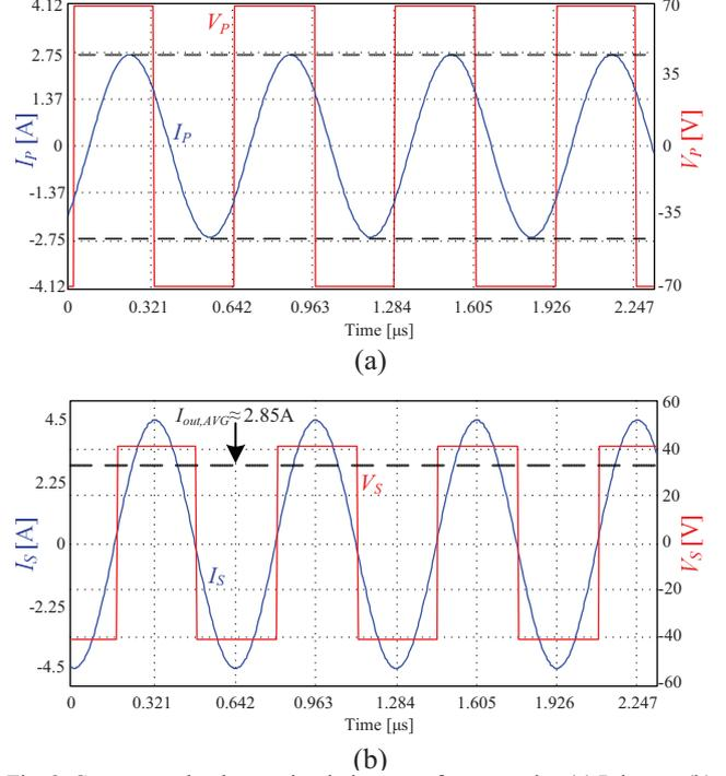
Fig. 8. Currents and voltages simulation waveforms results: (a) Primary, (b) Secondary.
