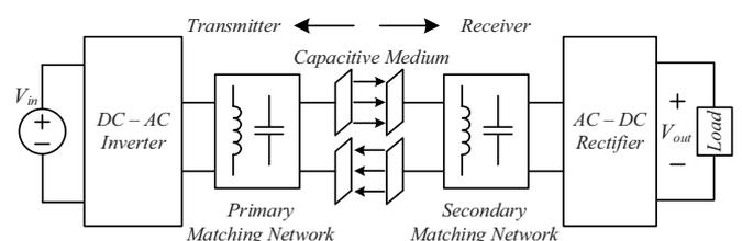
Fig. 1. Typical diagram of capacitive WPT system.
