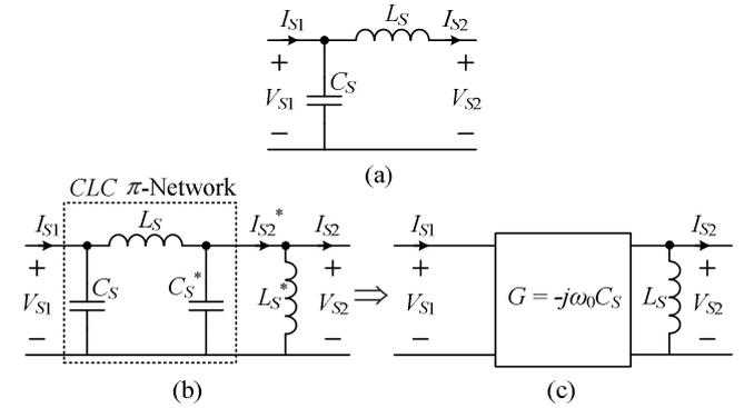
Fig. 4. Equivalent representations of parallel-series  $LC$  matching network: (a) L-type parallel-series resonant  $LC$  circuit; (b) Parallel resonator connected to the L-type circuit for  $\pi$ -type network arrangement; (c) Two-port representation of the original L-type network.
