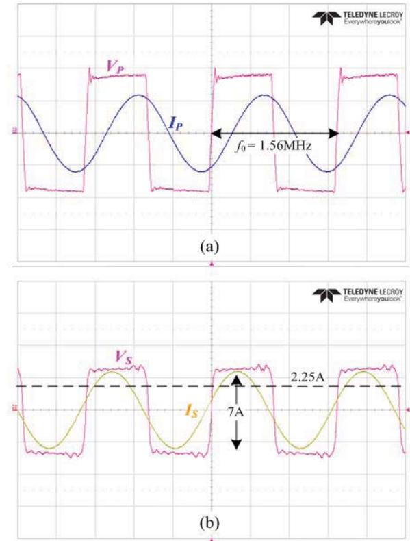
Fig. 11 Experimental waveforms with operating conditions:  $V_{in} = 70\text{V}$ ,  $R_{Load} = 15\Omega$ , coupling capacitance  $C_M \approx 6\text{pF}$ . (a) Primary side  $V_P$  40V/div,  $I_P$  3A/div, (b) Secondary side  $V_S$  20V/div,  $I_S$  3A/div. Time scale 200ns/div.
