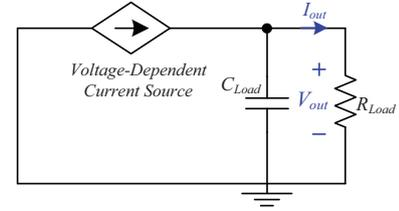
Fig. 7. Behavioral model of the analyzed capacitive WPT system.
