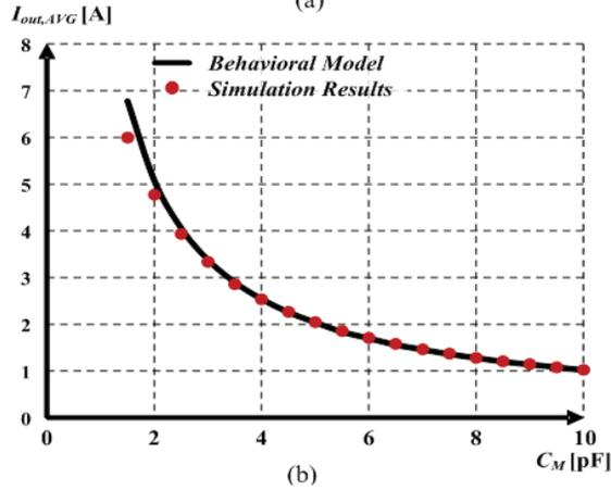
Fig. 9 Behavioral model and simulated average output current,  $I_{out,AVG}$ , curves: (a) As function of the input voltage  $V_{in}$ , (b) As a function of the mutual coupling capacitance  $C_M$ .
