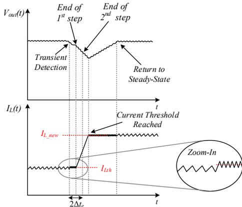
Fig. 3. Illustrative load estimation process for a loading transient when operating in constrained-current mode.
