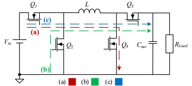
Fig. 2. Equivalent circuit of the non-inverting buck-boost converter in various stages of operation
