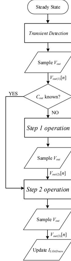
Fig. 4. Flowchart of the load estimation process
