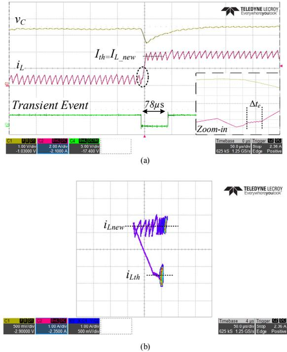
Fig. 8. NIBB converter's response and state-plane representation to a 0.8-3.6A loading event using current constrained controller and load estimation procedure in step-down configuration. (a) Output voltage (top-yellow) 1v/div, inductor current (middle - red) 2A/div, transient event (bottom - green), time scale 100us/div. (b) State-plane representation of inductor current and output voltage.
