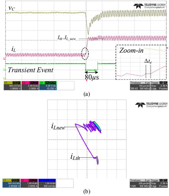
Fig. 7. NIBB converter's response and state-plane representation to a 0.8-2.9A loading event using current constrained controller and load estimation procedure in step-up configuration. (a) Output voltage (top-yellow) 500mv/div, inductor current (middle - red) 2A/div, transient event (bottom - green), time scale 100us/div. (b) State-plane representation of inductor current and output voltage
