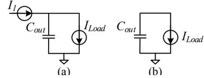
Fig. 5. Equivalent circuits of the converter. (a) step 1 operation. (b) step 2 operation.
