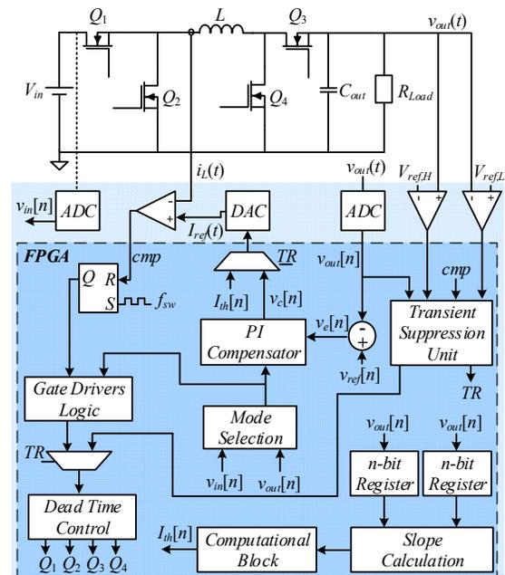
Fig. 1. Simplified schematic diagram, of a non-inverting buck-boost converter with current-programmed controller and the dedicated load-estimation blocks.
