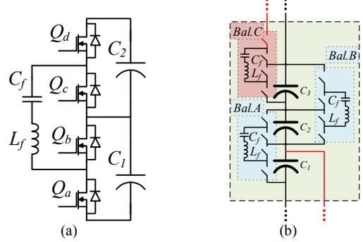
Fig. 3: Balancing circuits: (a) A single balancer schematic; (b) Balancers extra hardware for multimodule compatibility (balancer C and traces highlighted in bold red).
