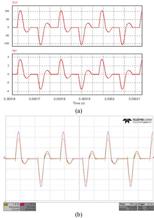
Fig. 6: Transformer resonant currents experimental vs. simulation results. (a) Simulation: primary current (top) 50A/div., secondary current (bottom) 2A/div.; (b) Experimental results: primary current (pink) 10A/div., secondary current (yellow) 0.5A/div.
