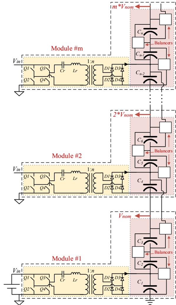
Fig. 1: Multilevel high voltage modular capacitor charger
