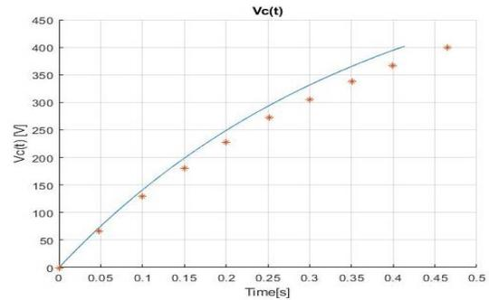
Fig. 12: Theoretical results of a single module charging times versus targeted output voltage with 3 capacitors in series,  $330\mu\text{F}$  each. Blue trace is a model calculation, and discrete stars in red are the PSIM numerical simulation. Parameters are:  $V_{in}=12\text{V}$ ,  $N=50$ ,  $D=0.9$ ,  $C_{out}=990\mu\text{F}$ ,  $R=96\text{m}\Omega$
