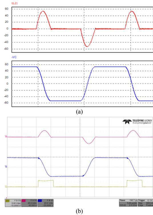
Fig. 9: Resonant capacitor  $C_r$  voltage and current in the middle of the charging process, at 60% point to target voltage: (a) Simulation results: from top to bottom: transformer primary resonant current 20A/div.,  $V_{Cr}$  20V/div., gate signal. (b) Experimental results: transformer primary resonant current (pink) 20A/div.,  $V_{Cr}$  (blue) 20V/div., gate signal ( $Q_2$ ) (yellow) 5V/div.
