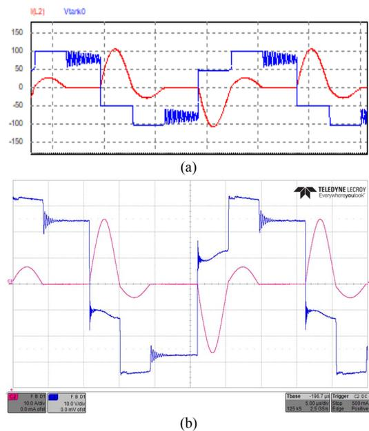
Fig. 7: Resonant tank voltage. Experimental vs. simulation results. (a) simulation results: transformer primary resonant current (red) 50A/div., resonant tank voltage (blue) 50V/div., (b) Experimental results: transformer primary resonant current (pink) 10A/div., resonant tank voltage (blue) 10V/div.
