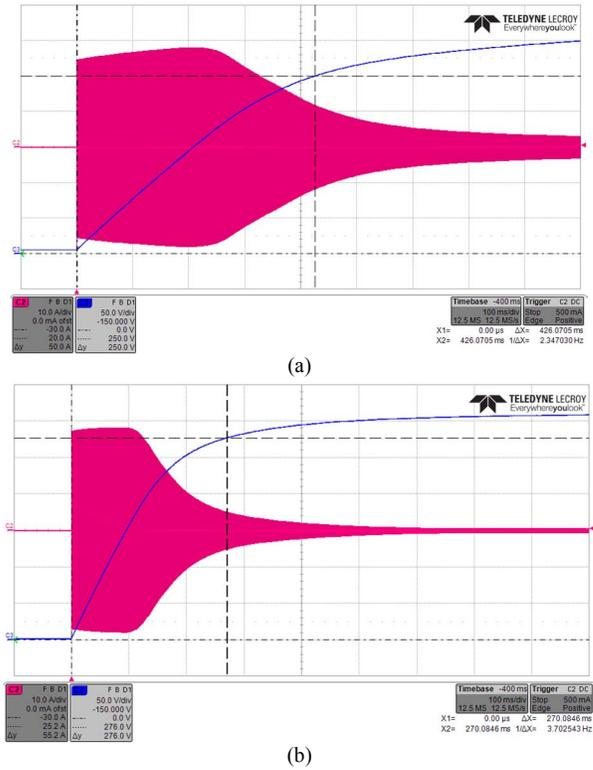
Fig. 11: Experimental results: full charge of output capacitor with  $C_{out}=330\mu\text{F}$ ,  $V_{in}=12\text{V}$ , Transformer primary resonant current (pink) 10A/div.,  $V_{out}$  on  $C_{out}$  (blue) 50V/div. with time scale: 100ms/div. (a)  $D=0.3$ ,  $P_{out\_avg}=25\text{W}$ ,  $P_{out\_max}=70\text{W}$ , (b)  $D=0.6$ ,  $P_{out\_avg}=45\text{W}$ ,  $P_{out\_max}=140\text{W}$
