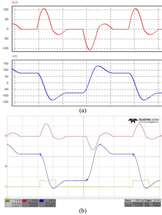
Fig 8: Resonant capacitor  $C_r$  voltage and current at the beginning of the charging process: (a) Simulation results: from top to bottom: transformer primary resonant current 50A/div.,  $V_{Cr}$  50V/div., gate signal. (b) Experimental results: transformer primary resonant current (pink) 20A/div.,  $V_{Cr}$  (blue) 20V/div., gate signal ( $Q_2$ ) (yellow) 5V/div.
