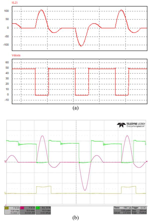
Fig. 10: Switch  $Q_5$  (keeping DCM operation) drain-source voltage. Experimental vs. simulation results. (a) Simulation results: from top to bottom: transformer primary resonant current 50A/div.,  $V_{DS-Q5}$  10V/div., gate signal. (b) Experimental results: transformer primary resonant current (pink) 10A/div.,  $V_{DS-Q5}$  (green) 10V/div., gate signal ( $Q_2$ ) (yellow) 5V/div.
