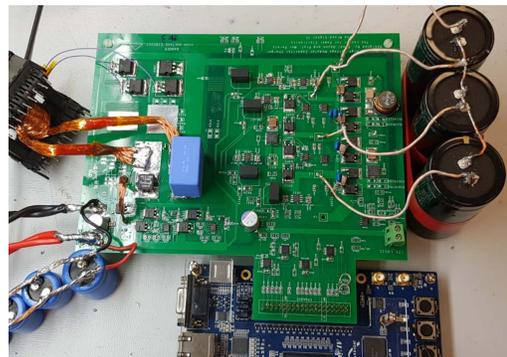
Fig. 13: Prototype board, including charger and balancer.
