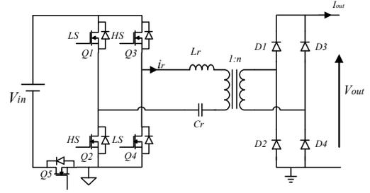
Fig. 2: Full bridge isolated capacitor charger
