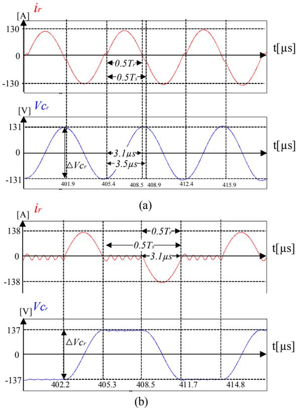
Fig. 5: Simulation of charging operation with: (a)  $D=0.9$ ; (b)  $D=0.5$ .
