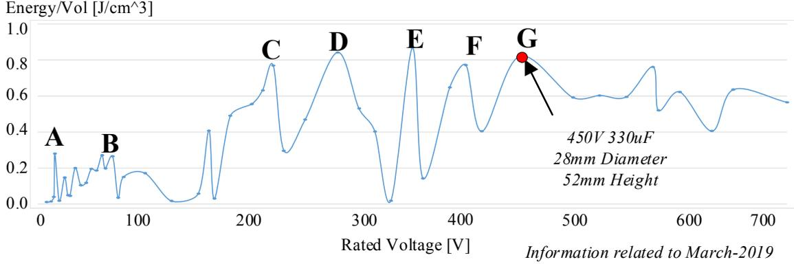
Fig. 4: Capacitor's energy density vs. maximum voltage rating
