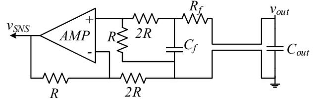
Fig. 5. Differential  $v_{out}$  sensing to single-ended interface.
