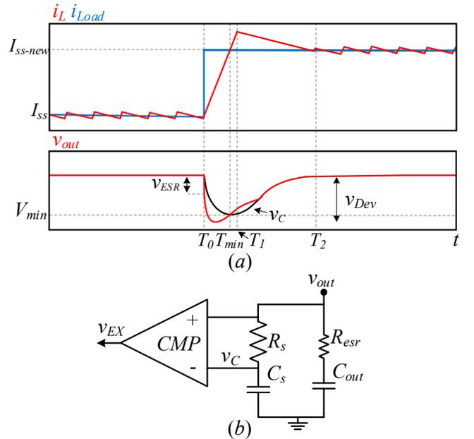
Fig. 2. (a) Typical waveforms of Time-Optimal recovery in single-phase buck for loading transient, with the presence of relatively high ESR. (b) Circuit for output capacitor voltage reconstruction and minimum voltage detection.
