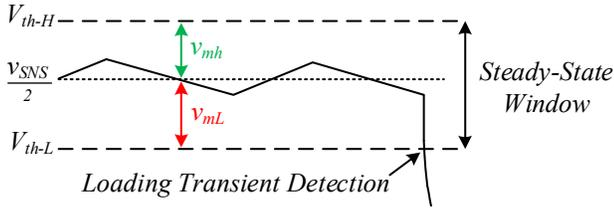
Fig. 7. Illustrative waveforms of window tracking and transient detection operation.
