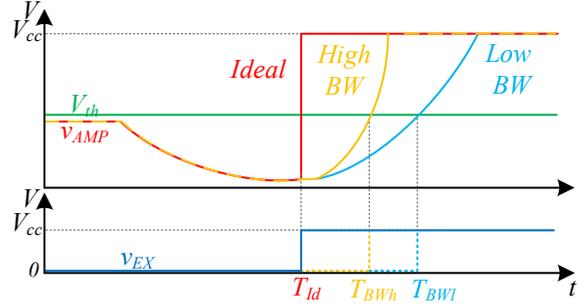
Fig. 9. Illustration of the impact of the sensor BW on the detection performance.
