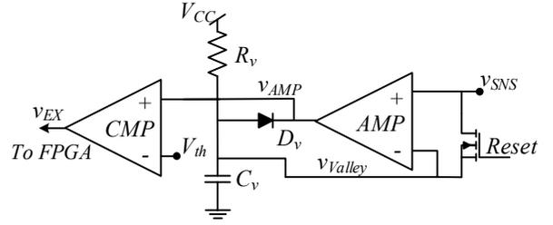
Fig. 8. Circuit description of extremum point detection; demonstrated for loading transients (valley point detection).
