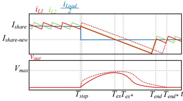
Fig. 3. Two phases interleaved buck converter operation with Time-Optimal Control during unloading transient. Recovery patterns for: (a) Synchronized operation. (b) Asynchronous, all-aligned ramp down.
