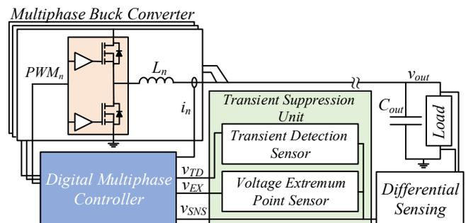
Fig. 1. Simplified schematic diagram of a multiphase buck system.
