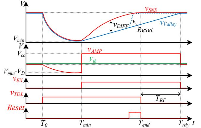
Fig. 4. Operation of the transient mitigation unit describing loading transient recovery.
