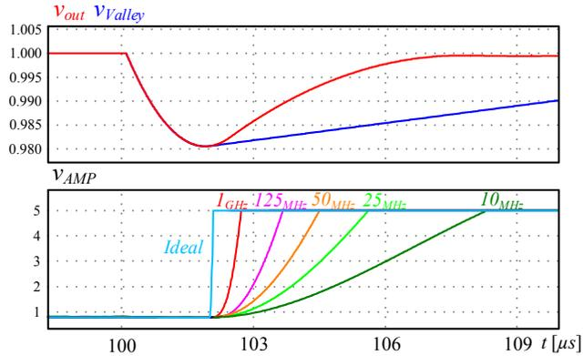
Fig. 11. Effect of sense amplifier bandwidth on extremum point detection.
