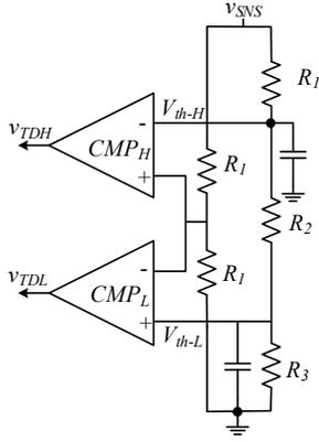
Fig. 6. Output voltage tracking window transient detection circuit.
