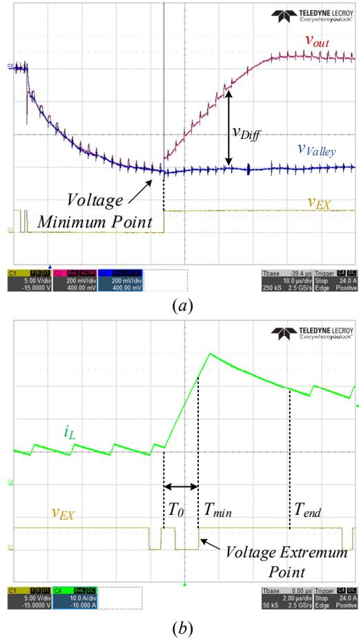
Fig. 12. Transient mitigation unit experimental results (a) two-phase multiphase buck converter 10A  $\rightarrow$  64A loading transient output voltage waveform (b) single phase operation 10A  $\rightarrow$  30A loading transient current waveform.
