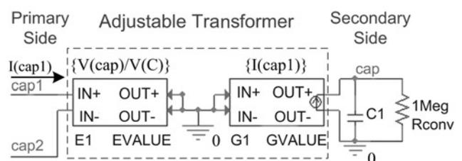
Fig. 3 Variable capacitor implementation in OrCAD PSpice
