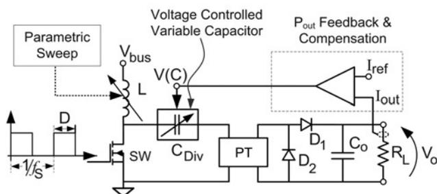
Fig. 2 Simulation scheme used to lower the number of unknowns from two to one
