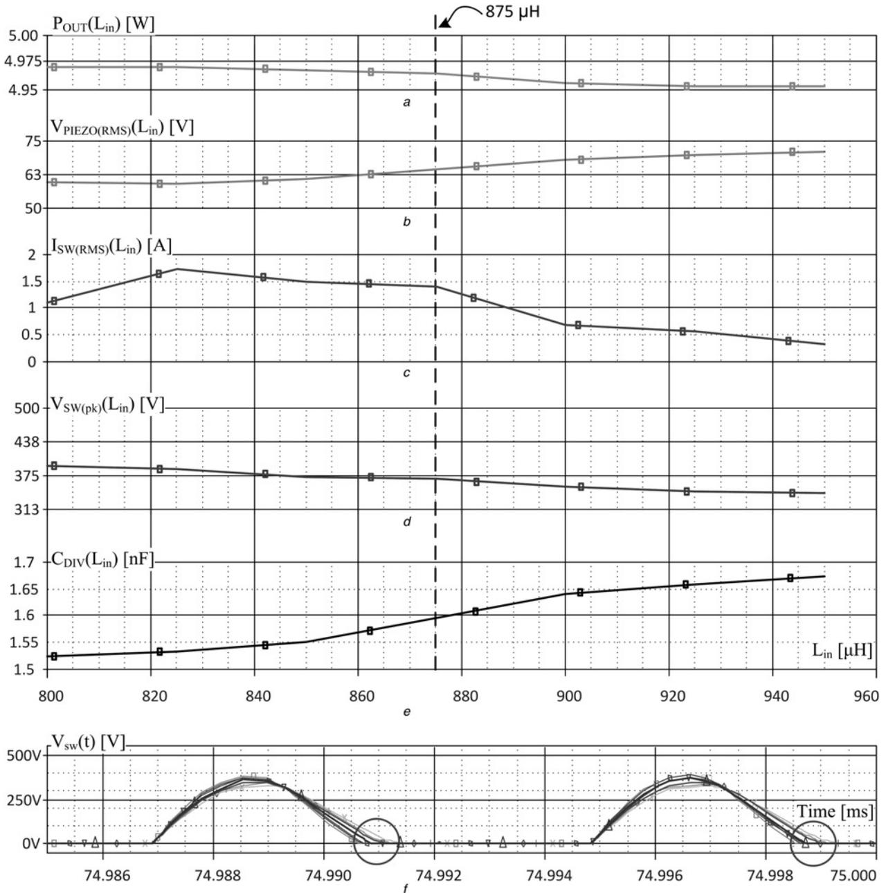
Fig. 5 Simulation results of driver optimisation procedure. Performance analysis (x-axis is an inductor value)
