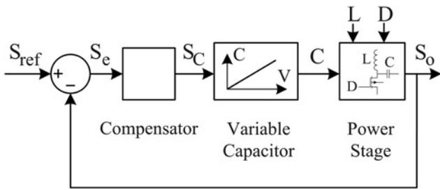
Fig. 4 Automatic capacitance adjustment control diagram
