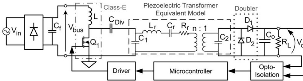
Fig. 1 Class-E converter with PT represented by its equivalent model
