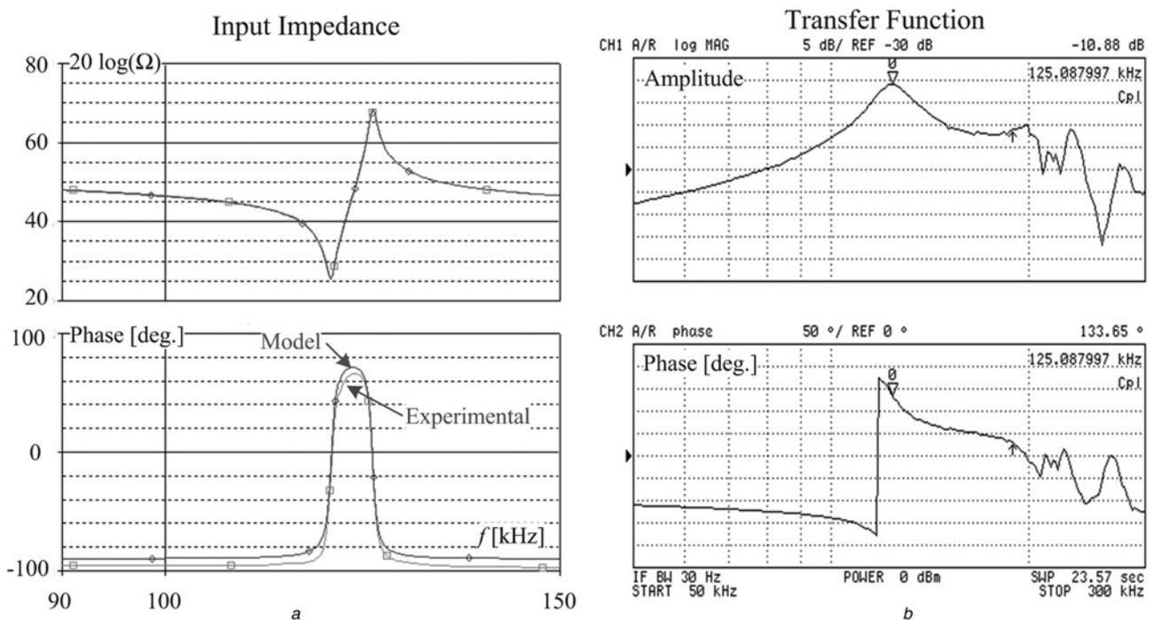
Fig. 7 Experimental results – response of the bare PT element
