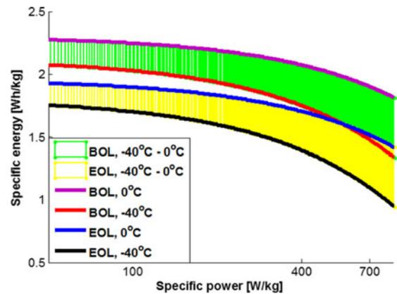
Fig. 3. Two-dimensional Ragone plot for different age and temperature conditions.
