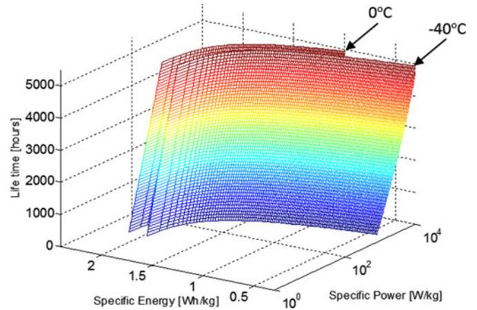
Fig. 2. Three-dimensional Ragone plot for different age and temperature conditions.
