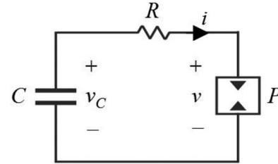
Fig. 1. SC connected to a power load.
