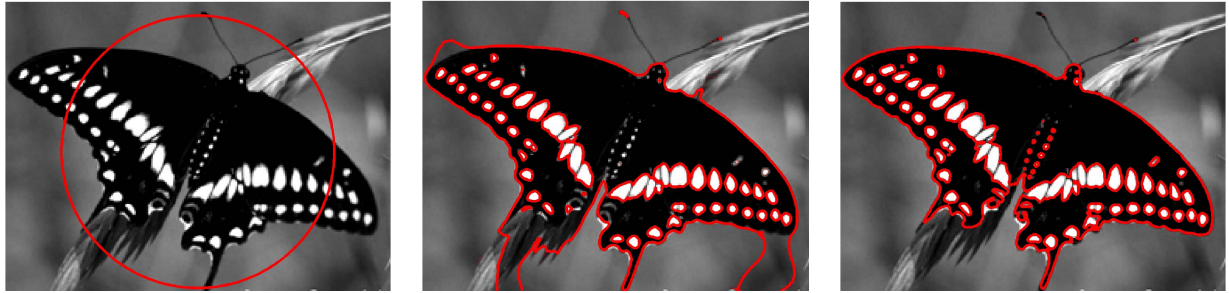
Figure 4. (a) Input image of a roughly symmetrical object with the initial segmentation contour (red). (b) Segmentation (red) without the symmetry constraint. (c) Successful segmentation (red) with the proposed algorithm. Original image courtesy of George Payne. URL: http://cajunimages.com
