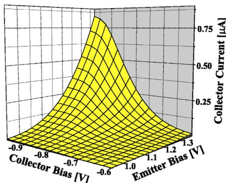
FIG. 2. Injected hot hole collector current as a function of the emitter and collector voltage biases for the ballistic Hole Emission luminescence device at 77 K.
