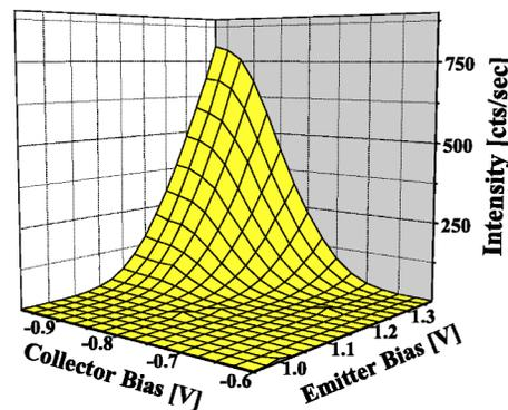
FIG. 4. Ballistic hole emission luminescence peak heights measured simultaneously with the data presented in Fig. 2. A collector bias threshold similar to the threshold seen in BEEL (Ref. 1) is evident.
