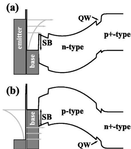
FIG. 1. Schematic band diagram for a BEEL device, (a), and for a BHEL device, (b). The emitter is shown biased, and the collector unbiased in both. In BEEL, the energy distribution of emitted electrons favors Schottky-barrier hot electron collection; this distribution makes hot hole injection in BHEL more difficult.
