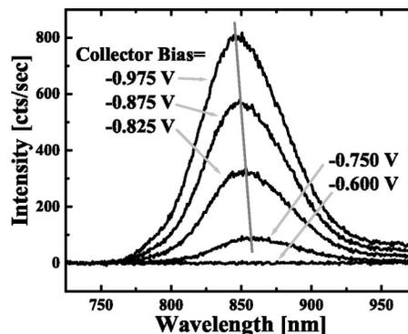
FIG. 3. Ballistic hole emission luminescence at constant emitter bias (1.375 V), for several collector biases at 77 K. The gray line indicates the blueshift caused by the  $V_{\text{collector}}$ -induced quantum-confined Stark effect.
