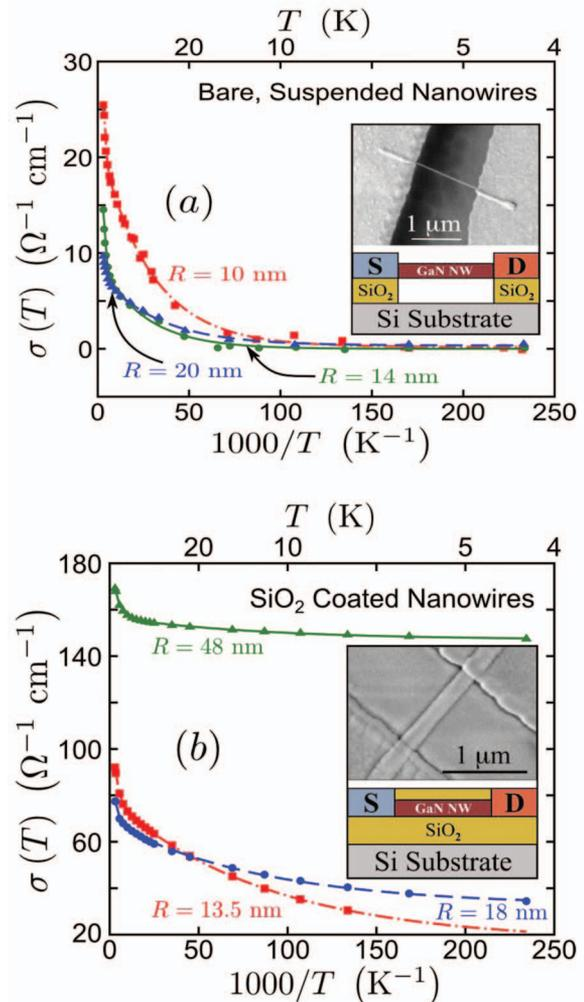
FIG. 1. (Color) The experimentally measured conductivity (points) and the fits to Eq. (1) (curves) for (a) bare suspended GaN nanowires with 10, 14, and 20 nm radii, and for (b) SiO<sub>2</sub> coated GaN nanowires with 13.5, 18, and 48 nm radii. Each inset shows an SEM image and schematic representation of the dielectric configuration.
