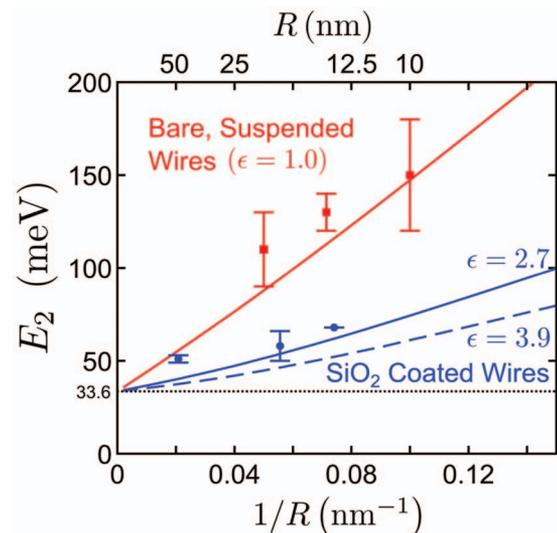
FIG. 2. (Color) The activation energies  $E_2$  (points) from fitting  $\sigma(T)$  with Eq. (1) for each nanowire vs the inverse wire radius, with the error in each energy. The curves are calculations from the FEM and were done with  $SiO_2$  dielectric constants of 2.7 and 3.9 for comparison, as the coating was not thermally grown and hence could have a dielectric constant different from that of bulk  $SiO_2$ .
