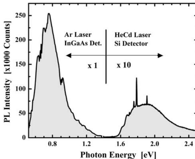
**Fig. 7** Room temperature photoluminescence, integrating emissions over a wide area, combining results of two measurements: One, with Ar laser pumping and InGaAs detector for the infrared range, and another using He–Cd laser pumping and Si detector for the visible range. It shows weak emission centered at 0.78 eV and even weaker emission peak centered at 1.9 eV
