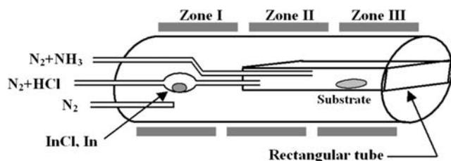
**Fig. 1** Horizontal HVPE reactor used for InN nanowire growth
