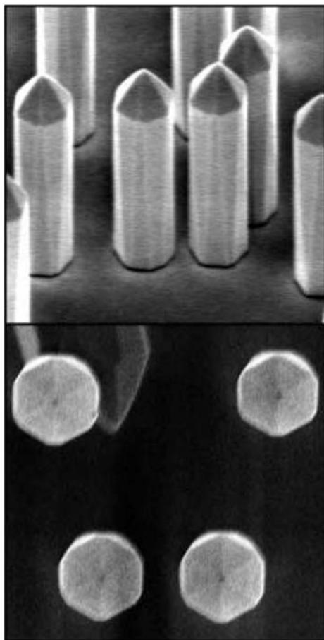
**Fig. 3** Vertical (top-panel) and rotational (bottom-panel) alignment between separate InN nanorods testifying epitaxial relations with the *c*-plane sapphire substrate. The top SEM image was taken at about 42° tilt. The bottom image was taken without tilt. Image width: top: 2  $\mu\text{m}$ , bottom: 1.5  $\mu\text{m}$
